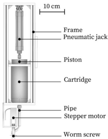
Figure 5. Schematic representation of the cartridge extruder.
